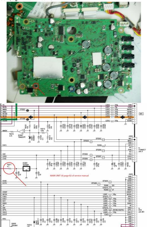
Ok, it looks like something else is shortening the output of that 7808. Traced the line and found it supplies power to the Display module (control head). One 7805 is there, checked and found ok. After checking all the capacitors found one of the big cap C502 is faulty. It is short. Removed it, checked everything else again.
